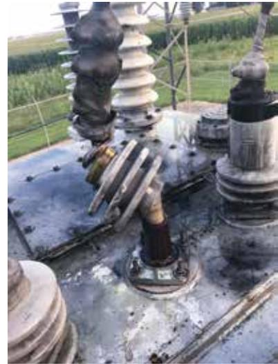
A close-up of the damaged transformer shows the bushing blown apart, with suspected damage also inside the transformer.
