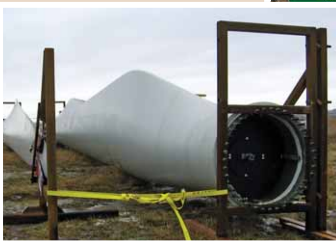
Two of the 80-foot blades wait to be assembled in December. They're several feet in diameter at the base, tapered down to a few inches thick at the other end.
