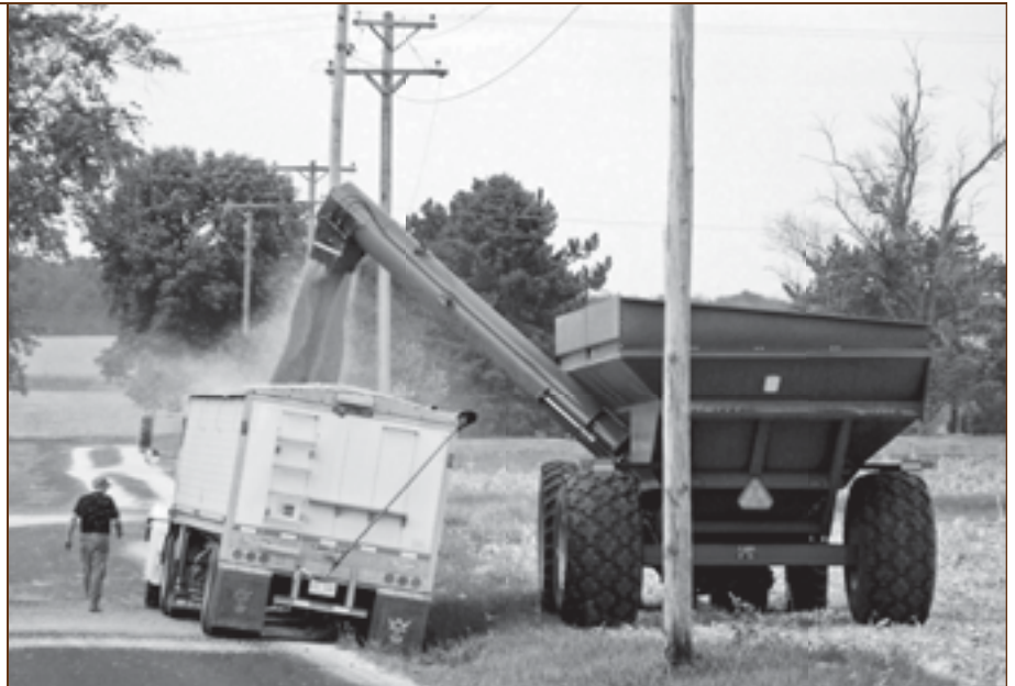
Large farm equipment should be kept away from overhead power lines to avoid possible contact.
